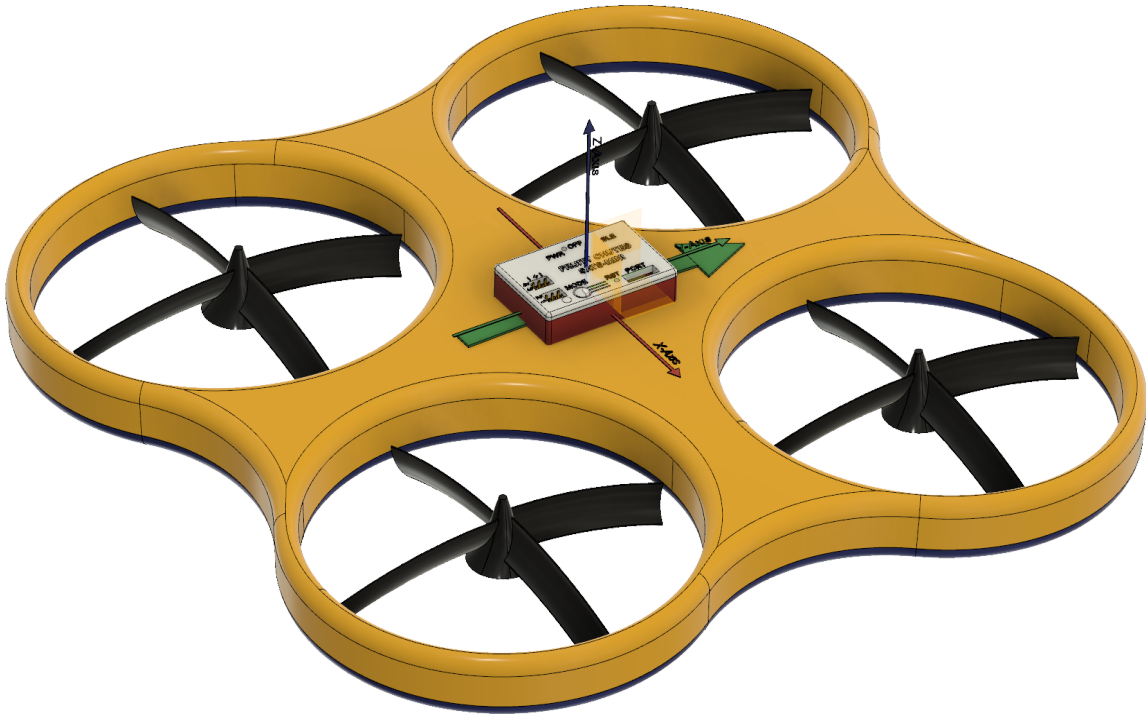
SATS-MINI Mounted Native Orientation at X:0, Y:0, Z:0
